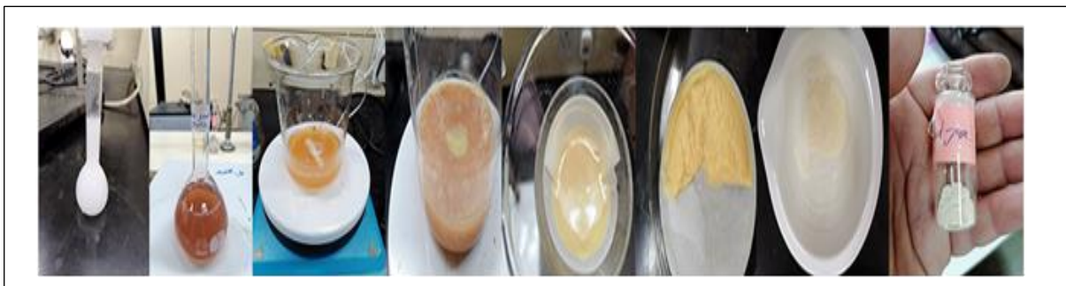
Figure 1: \text{TiO}_2\text{-NPs} green synthesis steps by the Sol-Gel method.
