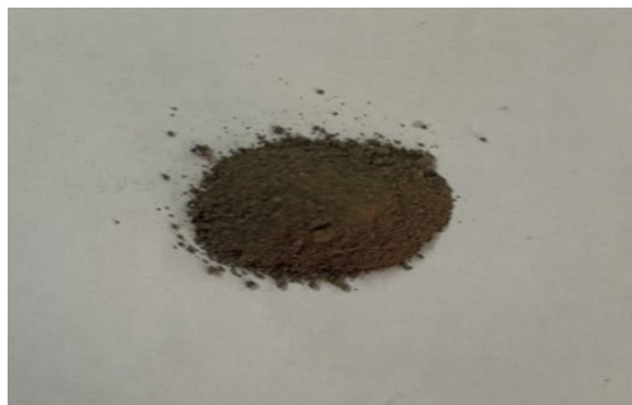
Figure 1: Zinc oxide nanoparticles, which were green synthesized from the aqueous extract of Ganoderma lucidum mushroom
