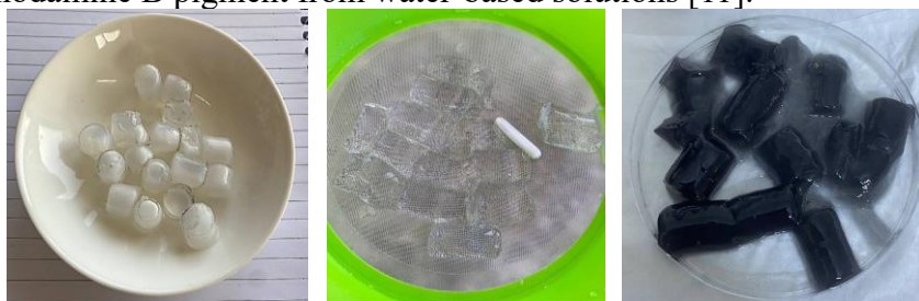
Figure 2: Polymer synthesis [PVA-g-P (AAM-co-MBA)]/Fe 3 O 4 /DES
