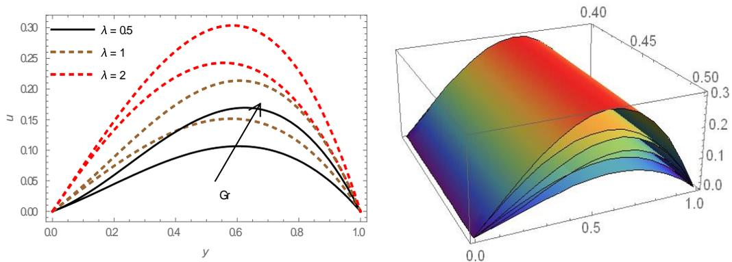
**Figure 3**-Velocity profile for  $\lambda$  and  $Gr$  with  $\omega = 1, N = 1, M = 1, Re = 1, Pe = 1, Da = 0.8, We = 0.05, t = 0.5$  in Poiseuille flow.
