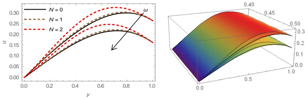
**Figure 10**-Velocity profile for  $\omega$  and  $N$  with  $Re = 1, Pe = 1, M = 1, \lambda = 1, Gr = 1, Da = 0.8, We = 0.05, V_0 = 0.3, t = 0.5$  in Couette flow.
