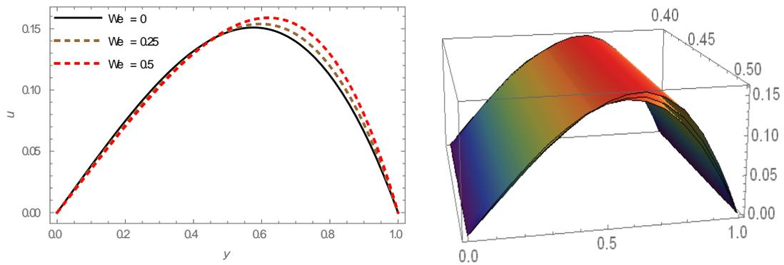
**Figure 6** -Velocity profile for  $We$  with  $\omega = 1, N = 1, Re = 1, Pe = 1, M = 1, \lambda = 1, Gr = 1, Da = 0.8, t = 0.5$  in Poiseuille flow.
