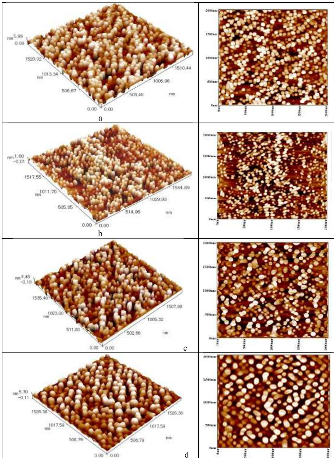
**Figure 5-**3D& 2D AFM images of (100:10) Alq<sub>3</sub>: C<sub>60</sub> / Si thin film at (a) as-deposited (b) Ta=373 K (c) Ta=423K (d) Ta=473K
