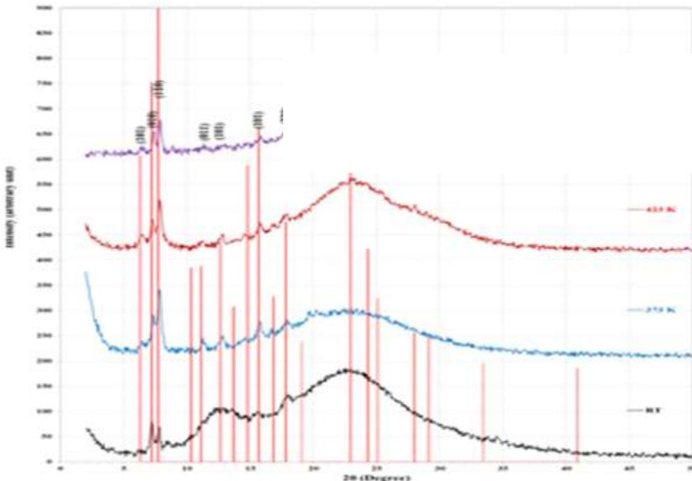
**Figure 3**-XRD pattern of as-deposited and annealing temperature blend (Alq<sub>3</sub>/ C<sub>60</sub>) thin films. (100:10).
