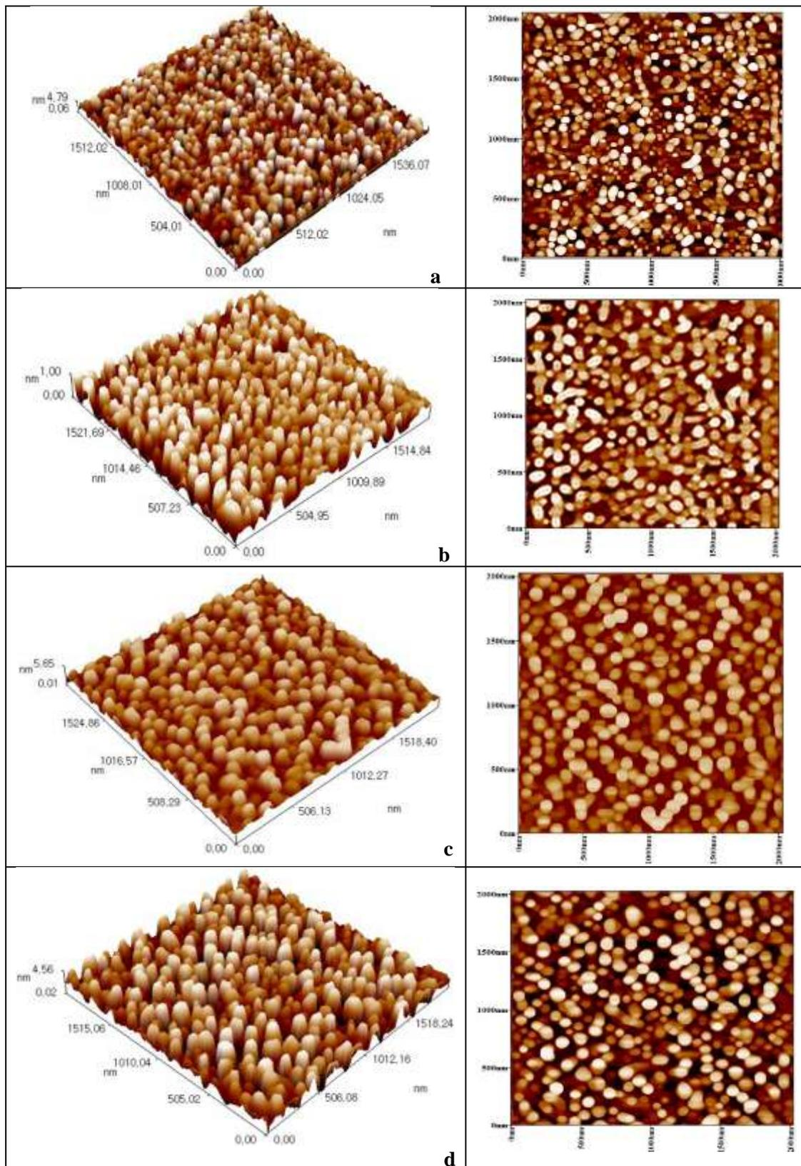
**Figure 7-**3D& 2D AFM images of (100:10) Alq3: C60 / PS thin film at (a) as-de posited (Ta=373 K (c) Ta=423K (d) Ta=473K
