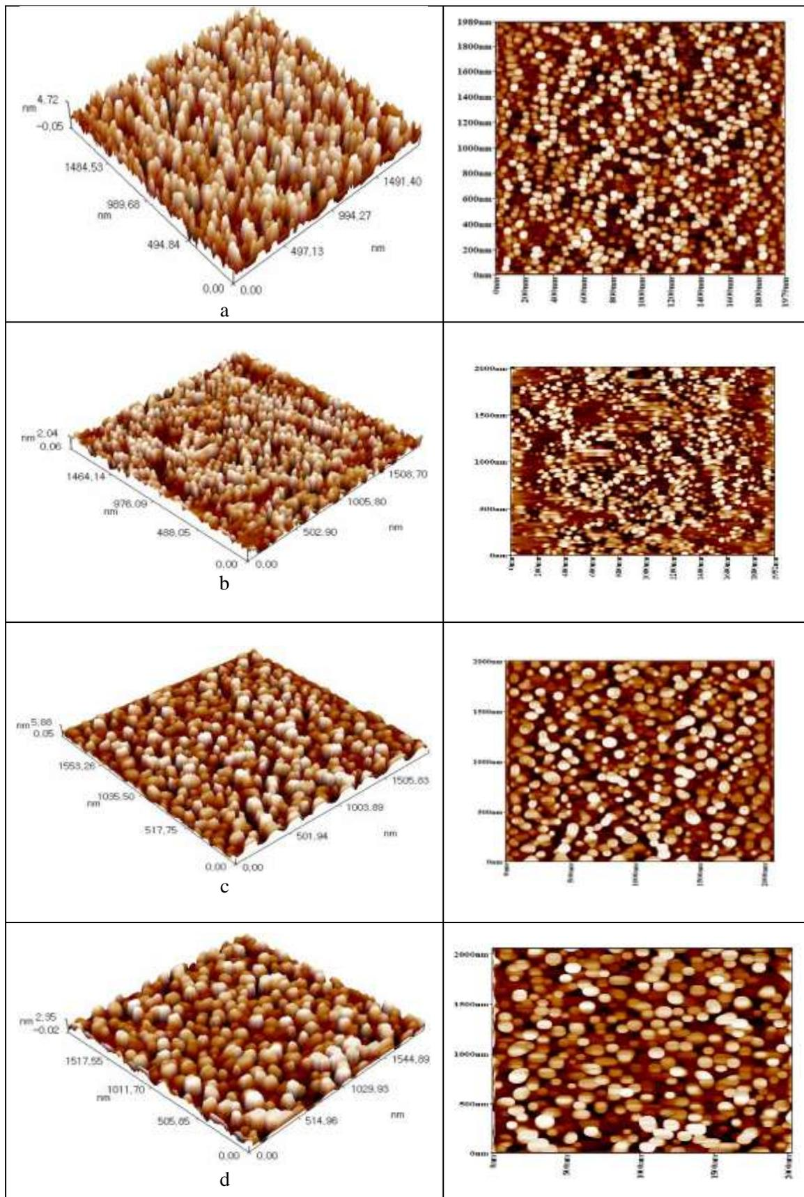
**Figure 4-**3D& 2D AFM images of (100:1) Alq3: C60 / Si thin film at (a) as-deposited (b) Ta=373 K (c) Ta=423K (d) Ta=473K
