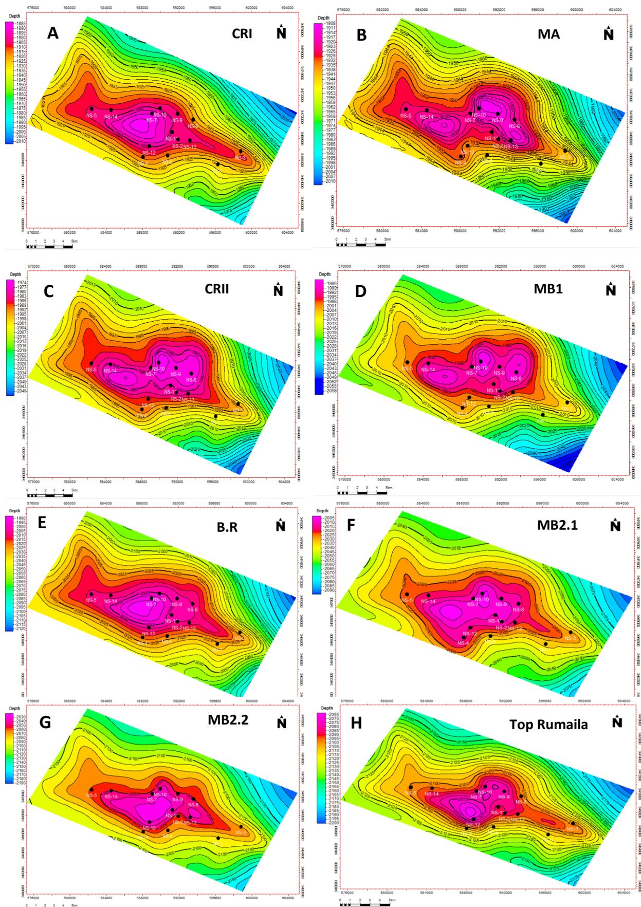
Figure 6- Shows the structural depth maps of Mishrif Formation units.
